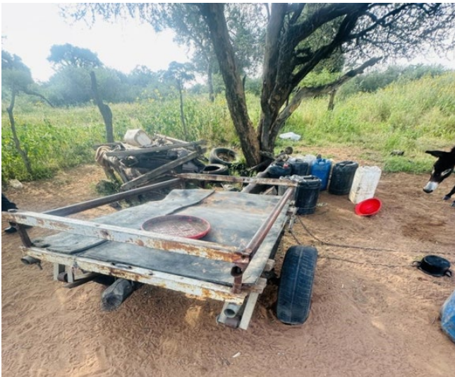
Recent picture of a cart made from vandalised transmission tower members.
