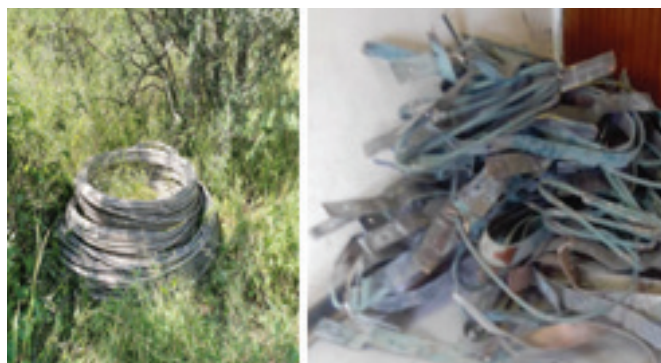
Figure 4: Stolen conductors and tower members in BPC, Botswana
